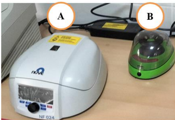
Figure 3.14. Shows two devices which used in this research, (A) microcenterfuge, (B) spin device
