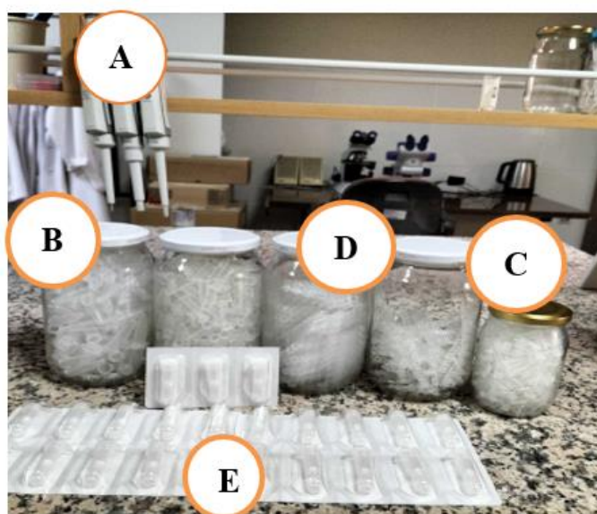
Figure 3.17. Shows some materials which were used in this study, A) pipetts in different sizes, B) Ependorf tubes 1.5 \mu l and 0.5 \mu l, C) PCR tubes 0.2 \mu l, D) PCR tubes and cups, E) filter tubes 2 \mu l (kit tubes)
