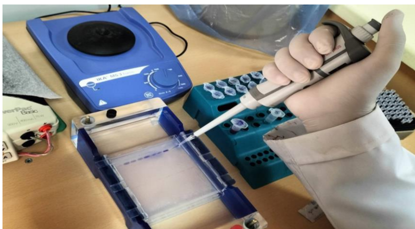
Figure 3.15. Loading 3 \mu l DNA with 3 \mu l bromophenol blue (loading dye) into wells of the 0.8-1% agarose gel
