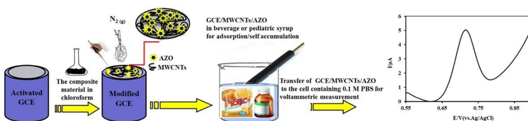
Figure 3.1. Preparation and use of GCE/MWCNTs/AZO
