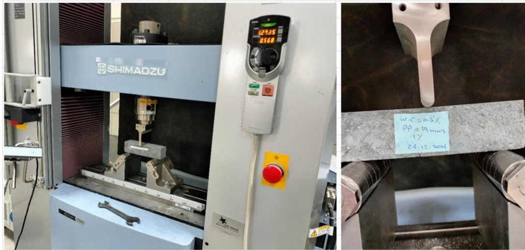
Figure 3.12. Photographic views from Harran University Laboratory: (b) Flexural strength test
