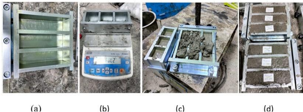
Figure 3.9. Photographic view of specimen preparation: (a) oiled molds, (b) empty mold weight, (c) finishing and Vibration machine and (d) Finishing and labeling
