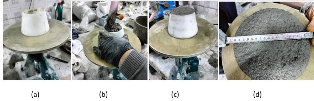
Figure 3.8. Flow Table Test for Fiber Mortar :(a) test apparatus, (b) filling & tramping stage, (c) finishing stage, and (d) measuring stage
