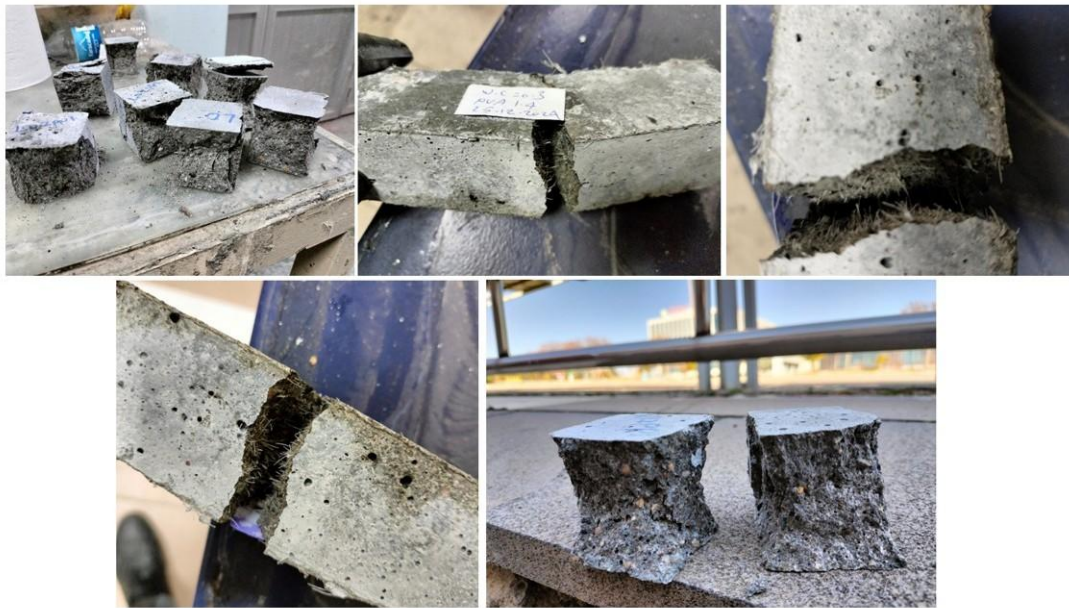
Figure 3.13. Photographic views from Harran University Laboratory: (c) Specimen shape after flexural failure indicating fiber pull-out and crack patterns and compressive samples show brittle fracture and crushed edges.
