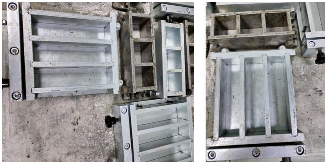
Figure 3.4. Molds used for production of test specimens
